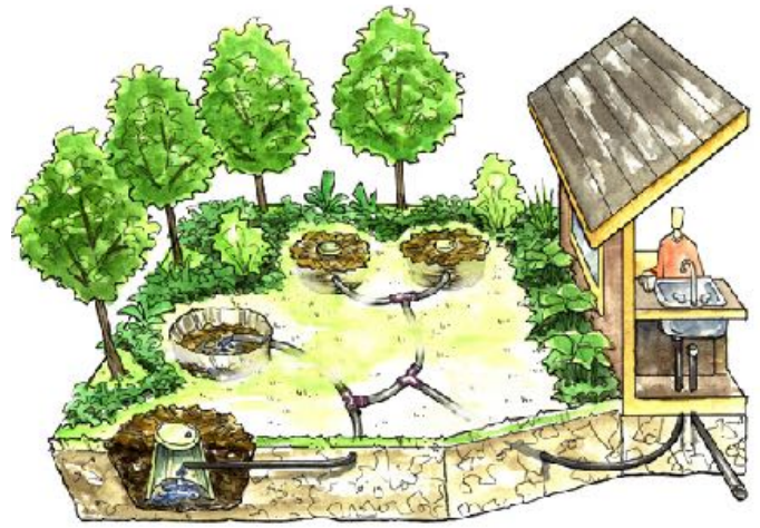
Figure 7: Illustration of a greywater landscaping system. Credit: Paul Kearsley
